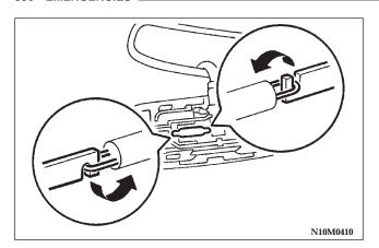
2. Remove the light bulb from the light holder.
